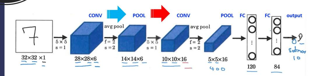
• Fill the table with the parameters corresponding to the figure of the LeNet-5 architecture (previous slide)
