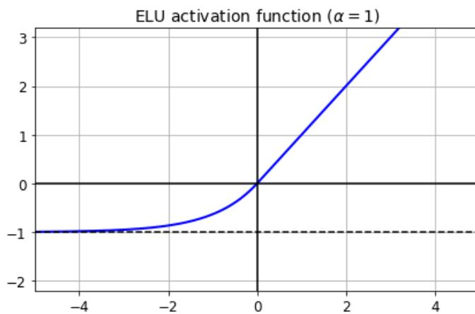
Implementing ELU in TensorFlow is trivial, just specify the activation function when building each layer:
